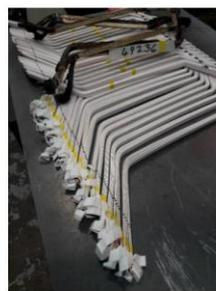
These sections of copper wiring are about to be put into one of the motors. They are a bit bigger than wires you will use for your Science experiments.
